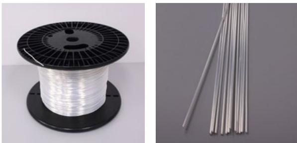
Film-coat PTFE liner is fabricated around a solid, silver-plated, copper-core mandrel. The mandrel remains in place throughout the catheter assembly process. It also helps maintain the surface quality of the PTFE liner, as tubing with only a 0.001" (0.025 mm) wall is susceptible to kinks and surface imperfections.
