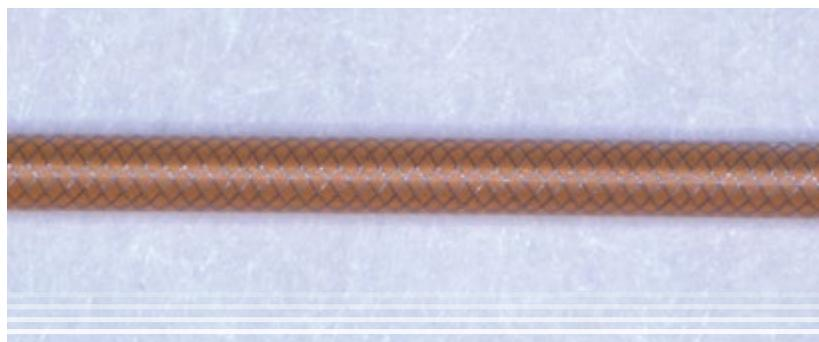
Thin-wall balloon delivery catheter. Wall construction = .0005" polyimide liner + .002" braid layer of .001" diameter round wire + .001" top coat of Pebax 72D.
